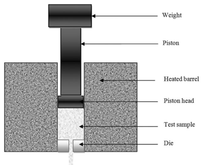
Figure 1: Schematic of MFI tester [9]
