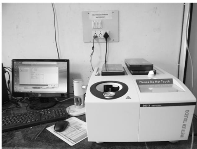
**Figure 2: Mettler Toledo DSC apparatus**
