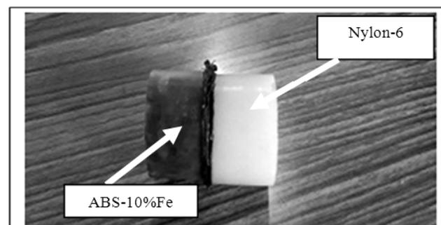
**Figure 3: Rotary friction welded joint of ABS-10%Fe and Nylon-6**
