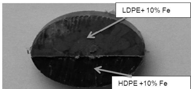
**Figure 4: Friction stir welded LDPE-10%Fe and HDPE-10%Fe**
