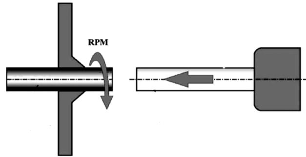
Figure 1: Mechanism for rotary friction welding [25]
