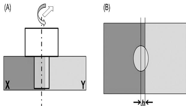
Figure 2: Schematic of friction stir welding (A), Top view of process (B) [21]
