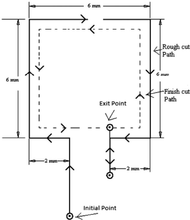
**Figure 1: Wire path profile during machining**
