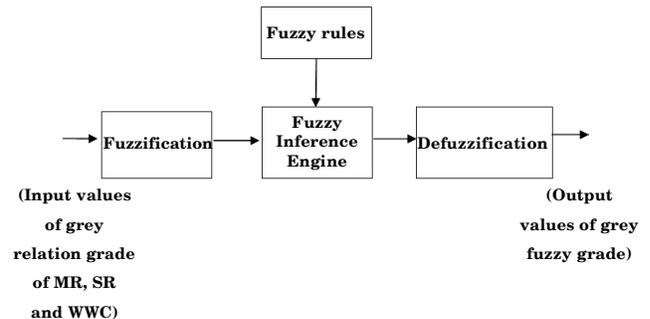
**Figure 2 Fuzzy logic mechanism**
