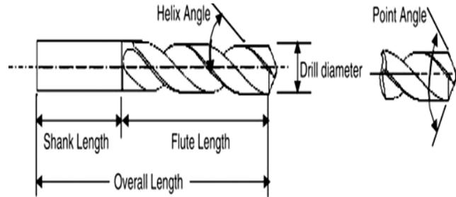
Figure 1: Geometry of twist drill consists of two flutes.
