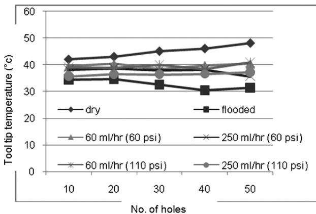
**Figure 3: Tool tip temperature generated during dry, flooded and MQL drilling at speed of 17.3 m/min.**
