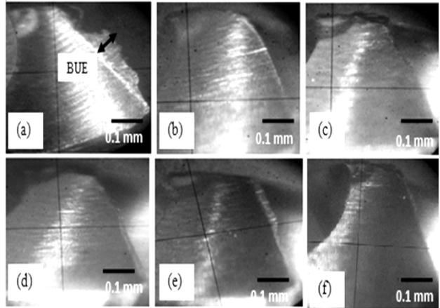
Figure 9: Optical micrographs showing the BUE (built-up edge) formation at the drill's cutting edge under different coolant-lubricant conditions at cutting speed 17.3 m/min. (a) Dry condition (b) Flooded condition (c) MQL {60 ml/hr at 60 psi} (d) MQL {60 ml/hr at 110 psi} (e) MQL {250 ml/hr at 60 psi} (f) MQL {250 ml/hr at 110 psi}.
