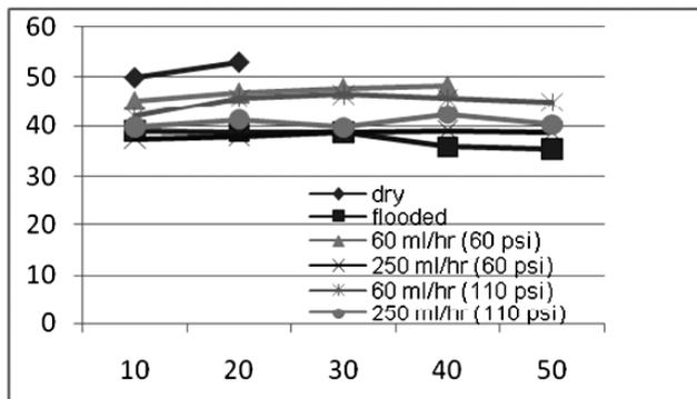
Figure 8: Hole temperature generated during dry, flooded and MQL drilling at speed of 53.7 m/min.
