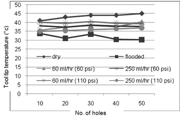
**Figure 4: Tool tip temperature generated during dry, flooded and MQL drilling at speed of 30 m/min.**
