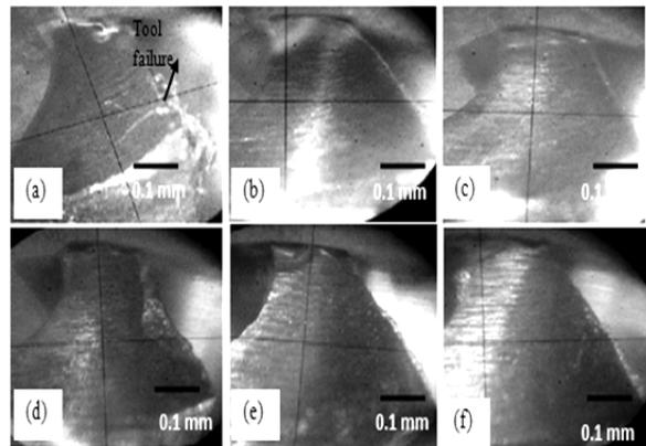
**Figure 11: Optical micrographs showing the BUE (built-up edge) formation at the drill's cutting edge under different coolant-lubricant conditions at cutting speed 53.7 m/min. (a) Dry condition (b) Flooded condition (c) MQL {60 ml/hr at 60 psi} (d) MQL {60 ml/hr at 110 psi} (e) MQL {250 ml/hr at 60 psi} (f) MQL {250 ml/hr at 110 psi}.**
