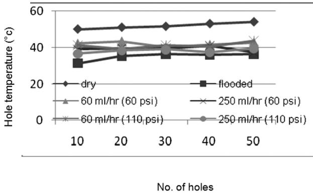
Figure 6: Hole temperature generated during dry, flooded and MQL drilling at speed of 17.3 m/min.
