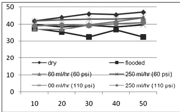
Figure 7: Hole temperature generated during dry, flooded and MQL drilling at speed of 30 m/min.
