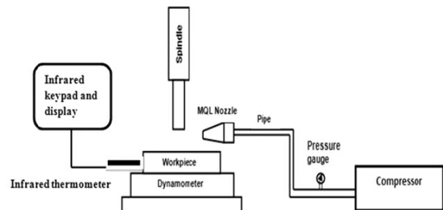
Figure 2: Schematic diagram of MQL drilling
