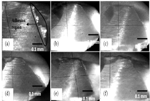
Figure 10: Optical micrographs showing the BUE (built-up edge) formation at the drill's cutting edge under different coolant-lubricant conditions at cutting speed 30 m/min. (a) Dry condition (b) Flooded condition (c) MQL {60 ml/hr at 60 psi} (d) MQL {60 ml/hr at 110 psi} (e) MQL {250 ml/hr at 60 psi} (f) MQL {250 ml/hr at 110 psi}.
