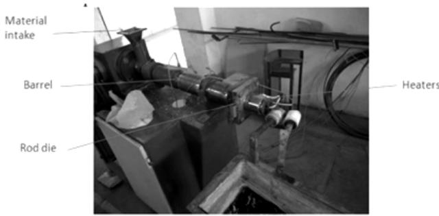
**Figure 5: Single screw extruder for extrusion of rods**
