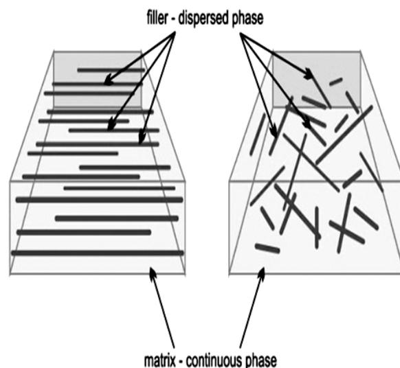
Figure 1: Schematic of a composite [1]
