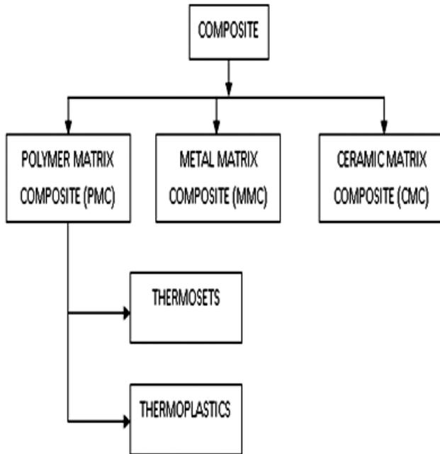
**Figure 2: Classification based on Matrix Material**
