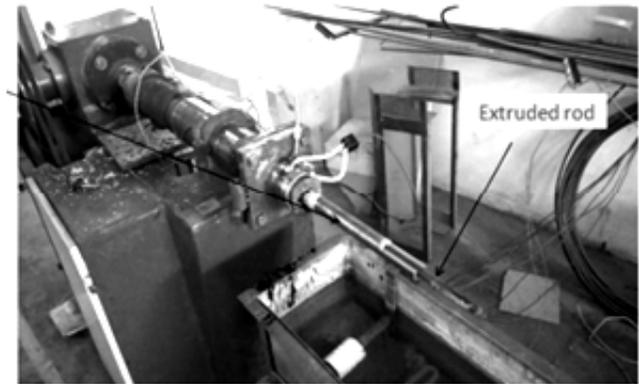
**Figure 8: Single screw extruder for extrusion of rods**
