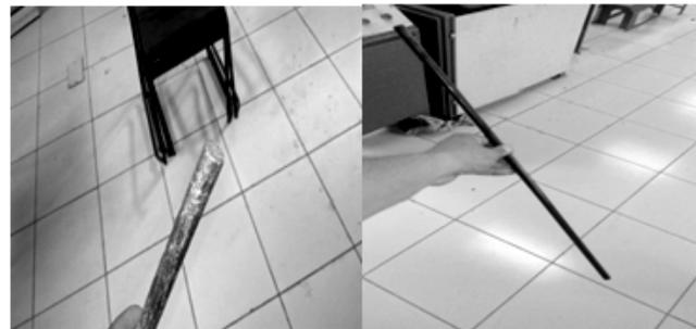
**Figure 9: Developed Green Rods. Only PLA (a) PLA and banana (b)**
