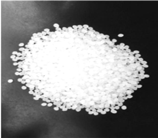
**Figure 6: Poly Lactic Acid in Granular form (3052D Injection grade)**
