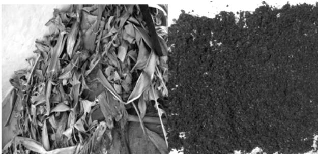
**Figure 7: Sunlight heat treated Banana leaves/stems and chopped banana fibres [a] Chopped fibers of Banana waste [b]**
