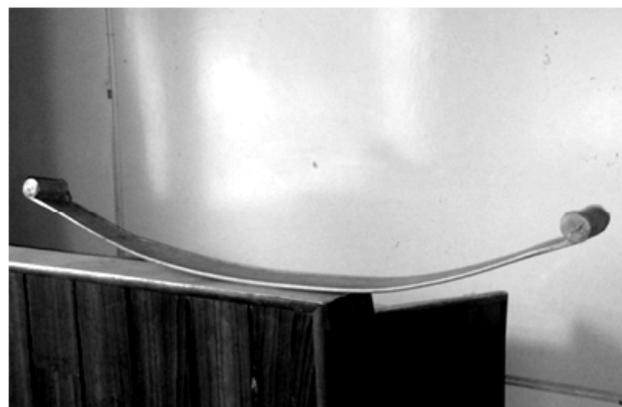
**Figure 1: Fabricated Al-B<sub>4</sub>C leaf spring**
