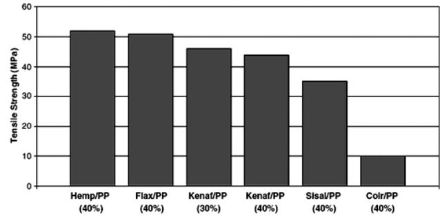
**Figure 4: Comparison of tensile strength of kenaf/PP-MAPP composite to other natural fiber composites[5].**
