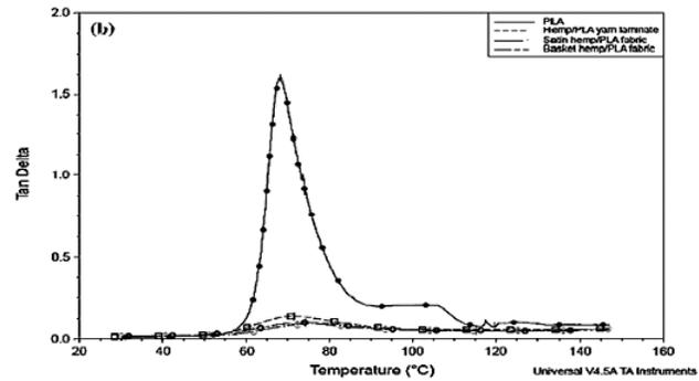
**Figure 9: DMTA analysis of thermoplastic PLA reinforced with of hemp fibre. Temperature vstan $\delta$  curves [15].**
