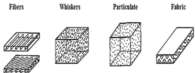
Figure 2: Schematic figure for understanding about Various distributions of fibers in polymer matrix.
