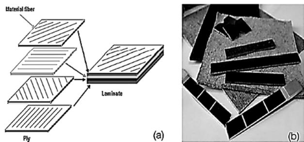
**Figure 7: (a) The vary of lay-up angles in the laminate; (b) resulted bio-composites [9].**
