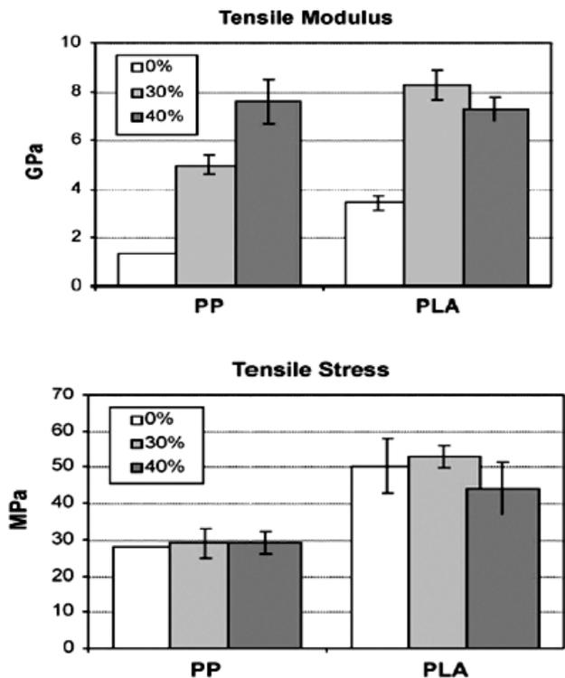
**Figure 5: Tensile stress and tensile modulus of PLA/flax composite compared with PP/flax[6].**
