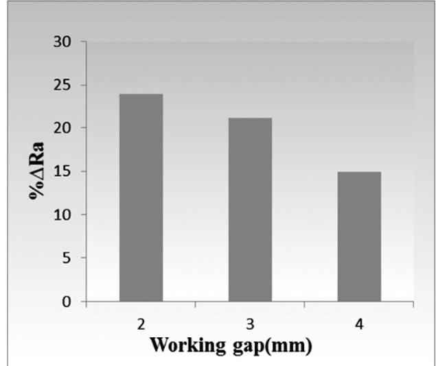
**Figure 1: Effect of working gap on surface finish with Micro abrasives**
