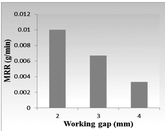
Figure 7: Effect of working gap on MRR with Nano abrasives
