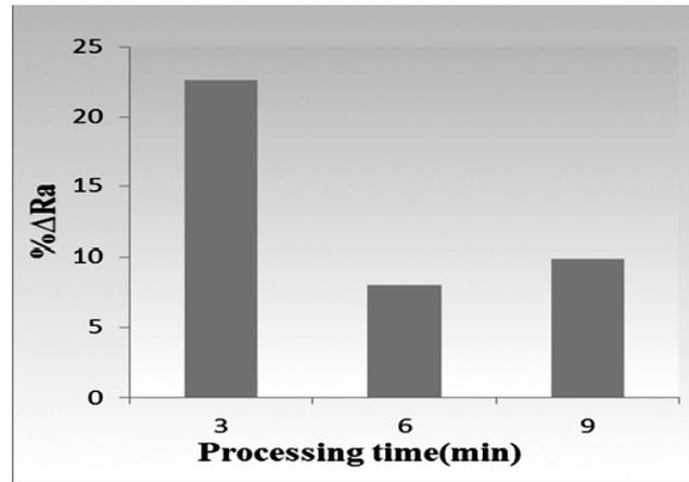
Figure 4: Effect of processing time on surface finish with Nano abrasives
