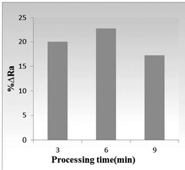
Figure 3: Effect of processing time on surface finish with Micro abrasives
