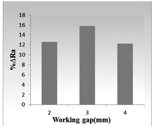
**Figure 2: Effect of working gap on surface finish with Nano abrasives**
